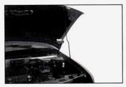
Before closing the hood, be sure all the filler caps are on properly. Then lift the hood to relieve pressure on the hood prop.
